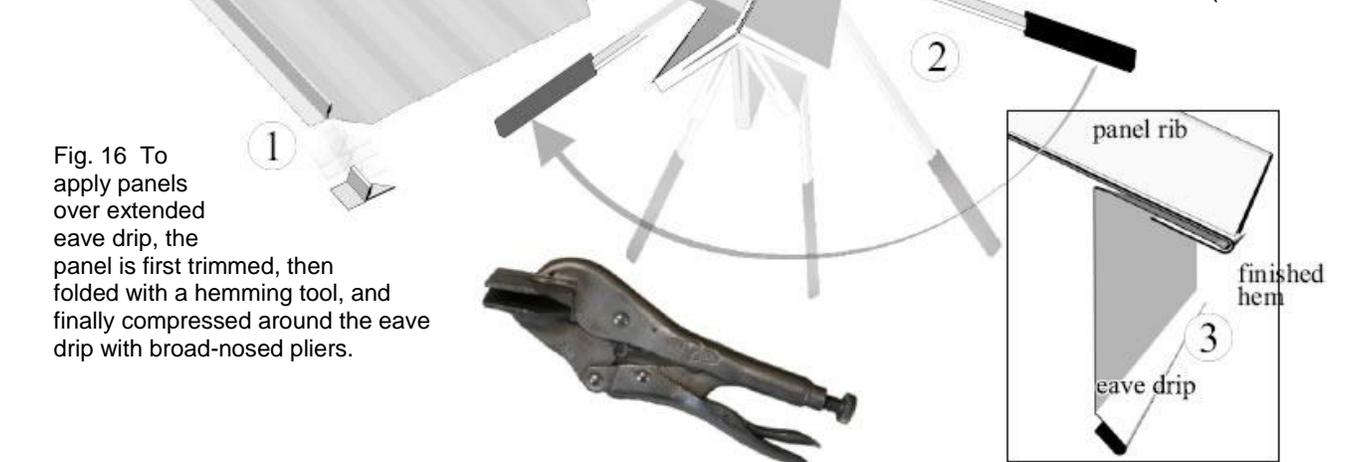
*Fig. 16 To apply panels over extended eave drip, the panel is first trimmed, then folded with a hemming tool, and finally compressed around the eave drip with broad-nosed pliers.*
